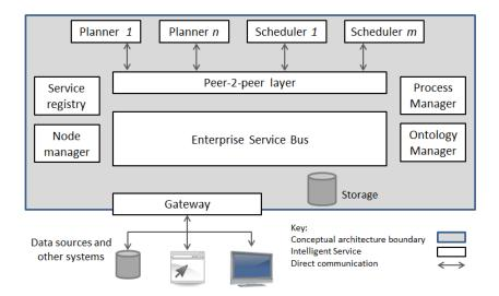
Figure 1. Intelligent Service based conceptual architecture iESB for supporting small lot production manufacturing.
