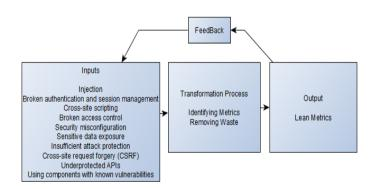
Fig. 5. Overview on security testing lean metrics finding.
