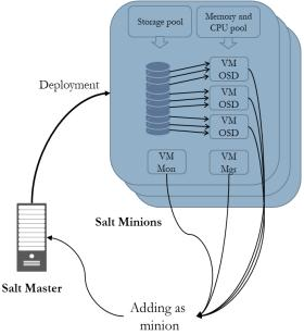
Figure 1. Deployment procedure for storage subsystem
