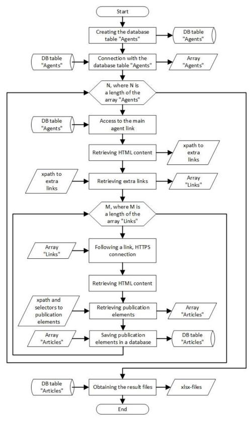
Figure 1. Algorithm for developing software for site monitoring
