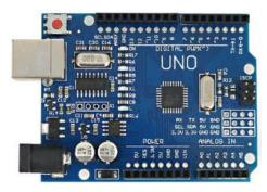
Fig 2 Arduino UNO with ATmega328p Microprocessor [28]
