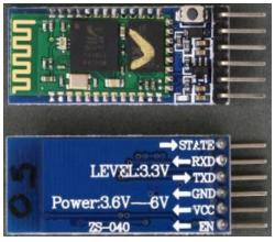
Fig 3. Fromt and Back view of HC-05 Bluetooth module [29]
