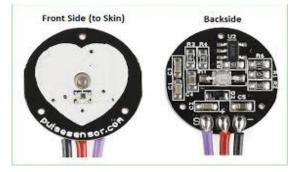
Fig 1. Front view and back view diagram of a pulse sensor [27]
