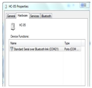
Fig 10: Port allocation to HC-05 Bluetooth module
