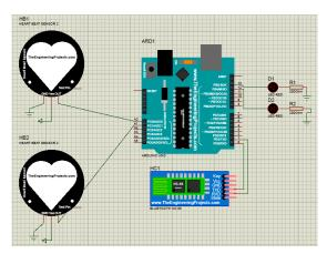
Fig 7: Block diagram of the remote heart rate monitoring system.
