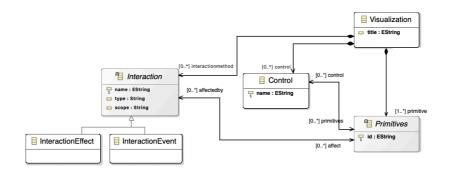
Fig. 1. Meta-model section regarding interaction patterns.
