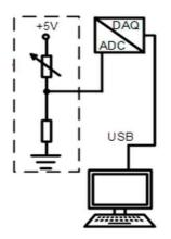
Figure 4. Voltage divider circuit [9]
