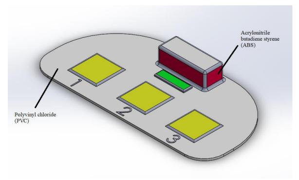
Figure 2. Design of the tactile mat.
