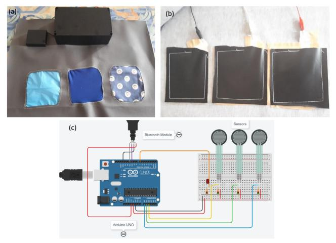
Figure 5. (a) Prototype of the device, (b) The Velostat of the tactile mat, (c) Circuit configuration
