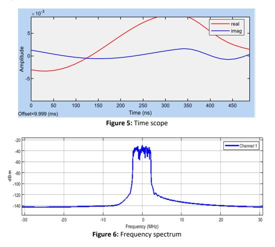
For QAM signal, the real and imaginary is represented on Fig. 7. The used filter is the root raised cosine with roll off is 0.3 with input bit is 60000.
