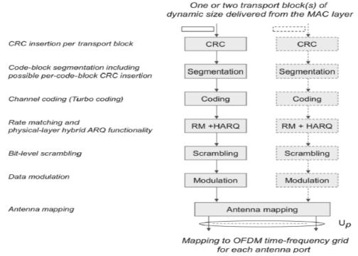
Figure 4: Processing of downlink Physical Layer
