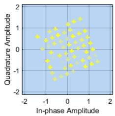
Figure 12: The constellation diagram of 64QAM at phase offset of pi/4 case
