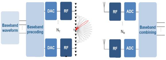
Figure 2: SDR and conversion from RF-baseband and vice versa
