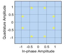
Figure 9: The constellation diagram of 8psk noiseless case
