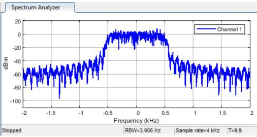
Figure 8: the frequency spectrum of 64QAM
