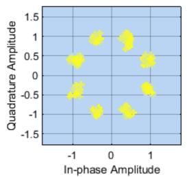
Figure 10: The constellation diagram of 8psk at AWGN case
