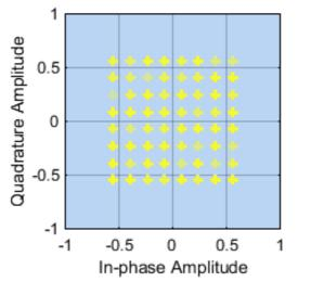
Figure 11: The constellation diagram of 64QAM noiseless case
